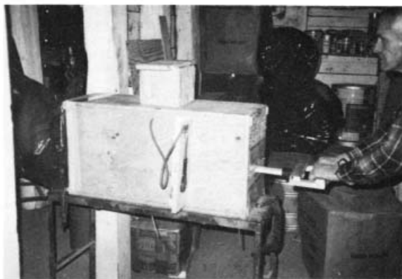
Fig. 1. Plywood Double-Action Piston Pump, with manometer attached for tests.
