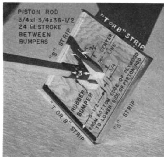
Fig. 14. Plywood Piston with Sheetmetal Sealing Strips Attached.
