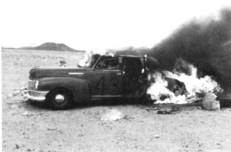
Fig. 7.2. Thermal radiation from a nuclear explosion entered the car above through its closed windows and ignited the upholstery. The windows were blown out by the blast a few seconds later. However, the explosion was at such a distance that the blast wave was not severe enough to dent the car body.
