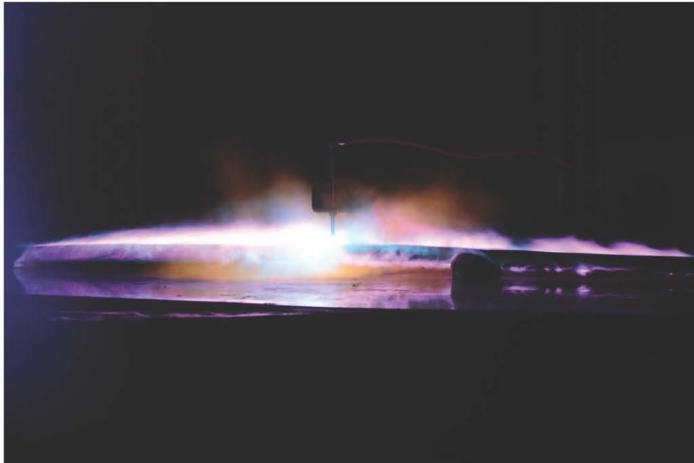
Fig. 3: Laboratory testing of CounterStrike with simulated lightning currents
